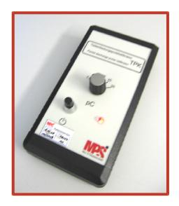
The **TPK** generates impulses of well known and constant charge with a repetition rate of about 100Hz. It is built in a handy housing and is battery-powered with a 9V battery.
