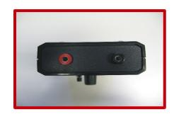
The output sockets are potential free. The black one is the reference output socket for getting positive impulses at the red socket. For calibration, the sockets must connected to the test circuit, the test object or the measuring instrument via short leads.
